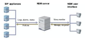
The IDP configuration, security policies, attack objects, and log records are stored in NSM server databases and administered using the NSM user interface. Communication between the NSM server and IDP appliances, and between the NSM server and the NSM user interface, is encrypted and authenticated.
